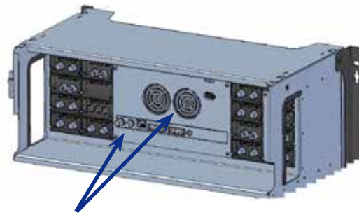
Remove all leads and cover panel
